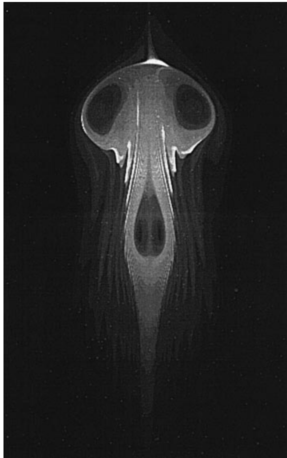
FIGURE 10. Visualized steady vortex-breakdown bubbles for H/R = 2.0 and Re = 1900 , first bubble diameter is 0.48R .
